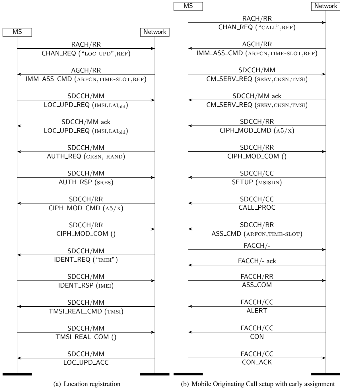
Figure 6.5: Scenarios showing actual message exchanges between MS and BTS
