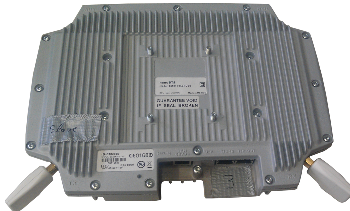
Figure 5.1.: nanoBTS with its antennas.
