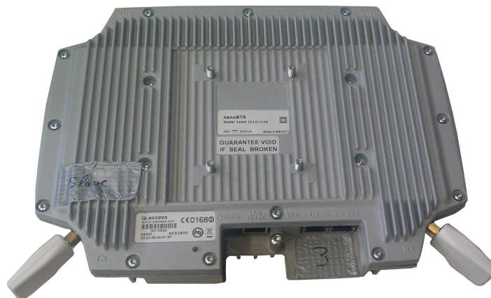
Figure 5.1.: nanoBTS with two external antennas and five connection ports
