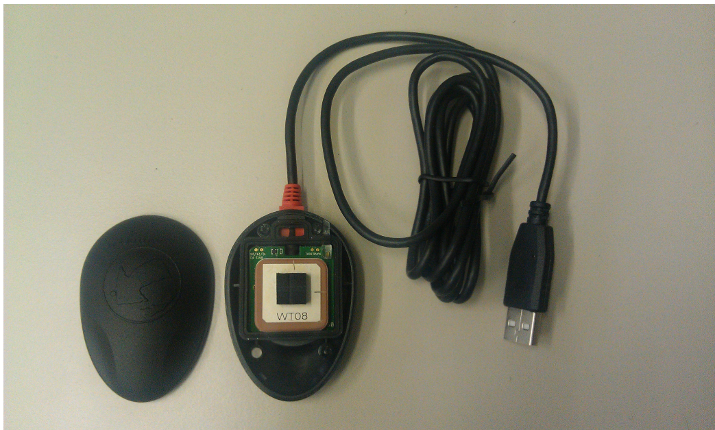
Figure 7.3.: Navilock NL-402U, opened up with the antenna and USB cable
