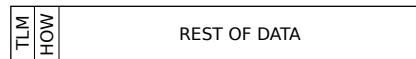
Figure 3.3.: Subframes always start with telemetry and handover words, the rest are parameters for removing errors and for estimating satellite's position.
