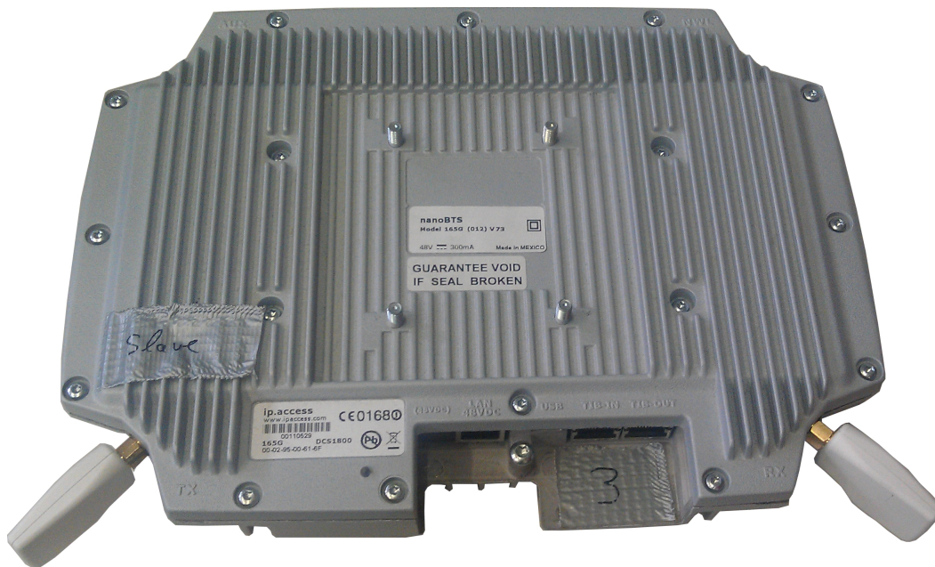
Figure 6.2.: nanoBTS with two external antennas and five connection ports
