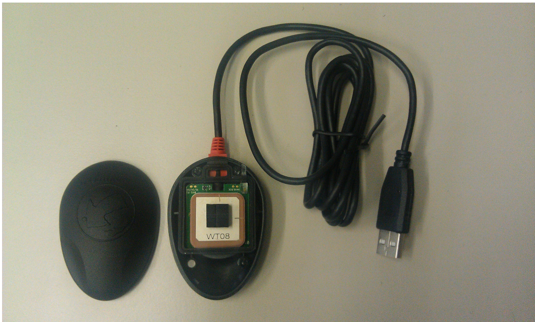
Figure 6.3.: Navilock NL-402U, opened up with the antenna and USB cable
