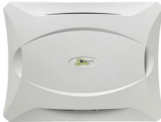
Figure 6.1.: nanoBTS with its plastic cover. Image courtesy of ip.access ltd
