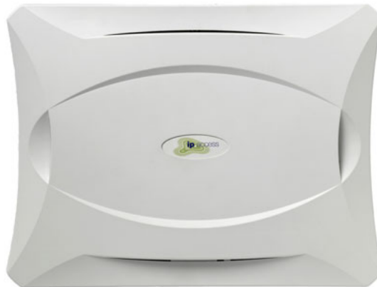
Figure 8.1.: nanoBTS with its plastic cover. Image courtesy of ip.access ltd
