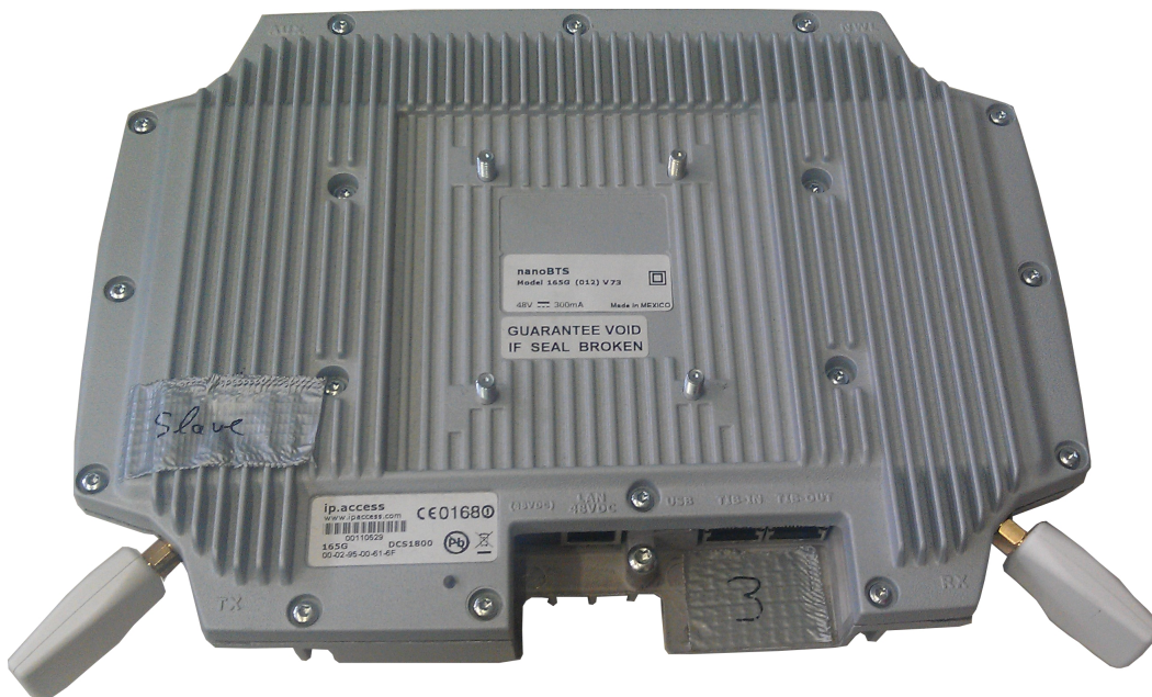
Figure 7.2.: nanoBTS with two external antennas and five connection ports
